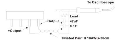
A 30cm twisted pair of no.18 AWG copper wire is connected to a 47uF and 0.1uF capacitor of proper polarity and voltage rating. The oscilloscope probe ground led should connect right to the ground ring of the probe and be as short as possible. The oscilloscope bandwidth should be at 20MHz and connected to AC ground.
