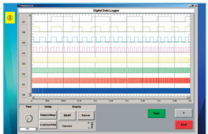
Windows software MEphisto Lab instrument soft-panels: ① Digital storage oscilloscope, time mode. ② Digital storage oscilloscope, XY mode. ③ Spectrum analyser. ④ Analog data logger. ⑤ Voltmeter. ⑥ Logic analyser. ⑦ Digital switchbox. ⑧ Digital data logger.
