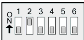
Figure 2.10. RS-485 (4-wire) and RS-422 DIP Switch Settings
