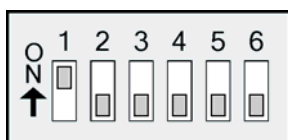
Figure 2.1. RS-232 DIP Switch Settings
